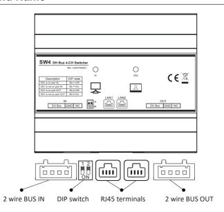
2 wire BUS in terminal: connect to 2 wire DH bus
